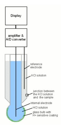
Calibration should be normally carried out using two standard buffer solutions that span the pH range for which the electrode is to be used. The clean and blotted dry electrode should be immersed in the buffer solution allowed to equilibrate and the pH meter adjusted to the known pH valueusing the calibration on the instrument. The process is the repeated with second buffer solution and any adjustment made using the slope and temperature.
